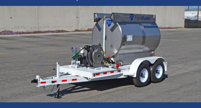
This package includes a 304 Stainless Steel DOT 406 Specification tank mounted on a 7K GVWR dual-axle steel trailer. The trailer is DOT-approved for use with Avgas, Jet-A, and JP-8. It can be towed on public highways when full, provided proper Hazmat placards and a commercial driver's license are obtained.
